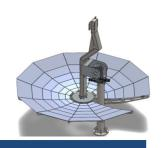
The Solar Energy Concentrator based on Stirling, CES-Stirling, harnesses solar energy through a circular paraboloid, which focuses sunlight onto a single point, the focus of the parabola. At this focal point, a thermal chamber delivers heat energy to the Stirling engine, which drives an alternator for the generation of 220/110 VAC electrical power.
